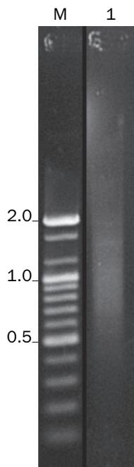
**Fig. 5. Result of agarose gel electrophoresis of cDNA that has been PCR amplified using a too-long extension step (6 min). No bright bands are visible, and a smear starting from the high-molecular-weight region of the gel is shown. Lane M – 1 kb DNA ladder.**
