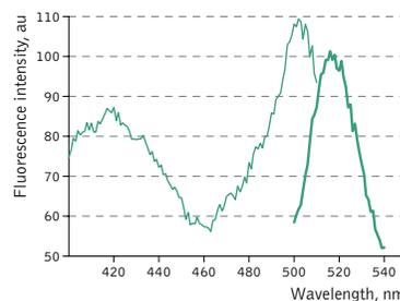
HyPer normalized excitation (thin line) and emission (thick line) spectra.
