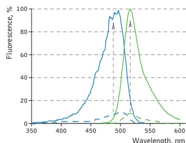
Case12 normalized excitation (blue line) and emission (green line) spectra without  $\text{Ca}^{2+}$  (dashed lines) and in the presence of 1 mM of  $\text{Ca}^{2+}$  (solid lines) [Souslova et al. 2007].
