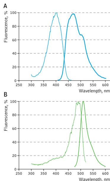
**PS-CFP2 normalized excitation (thin line) and emission (thick line) spectra.**
