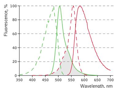
Excitation (dashed lines) and emission (solid lines) spectra of TagGFP (green) and TagRFP (red) are shown individually. Spectral overlap is filled with gray.
