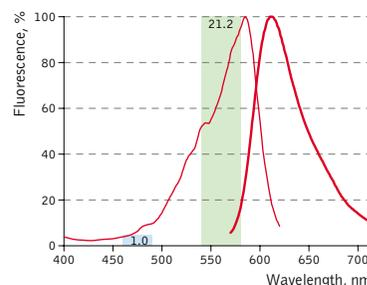
KillerRed normalized excitation (thin line) and emission (thick line) spectra.
