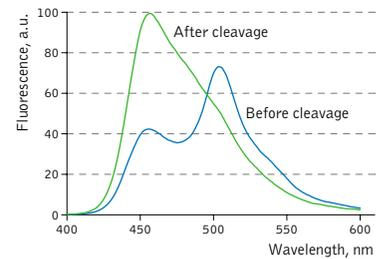
Change in Casper3-BG excitation/emission spectra upon the cleavage of DEVD sequence *in vitro*.
