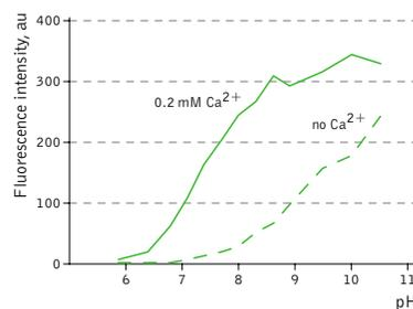
Dependence of Case12 fluorescence on pH in the presence (solid line) and in the absence (dashed line) of  $\text{Ca}^{2+}$  [Souslova et al. 2007].
