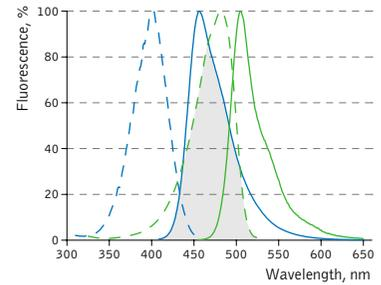
Excitation (dashed lines) and emission (solid lines) spectra of TagBFP (blue) and TagGFP2 (green) are shown individually. Spectral overlap is filled with gray.
